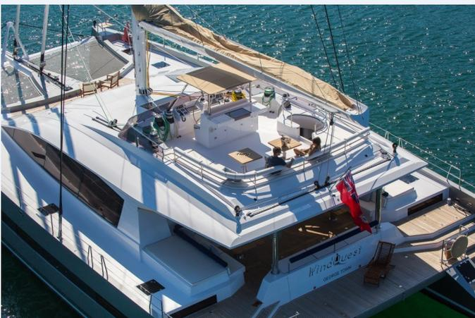
The hydraulic winches installed on the flybridge are well-suited to manoeuvring with a reduced crew. This yacht is equipped with 2 x 380HP engines and 2 x 27kW generators. At her economical speed, WindQuest motors at 8.6 knots for a fuel consumption of 21 l/h and can reach 12.9 knots at top speed.
