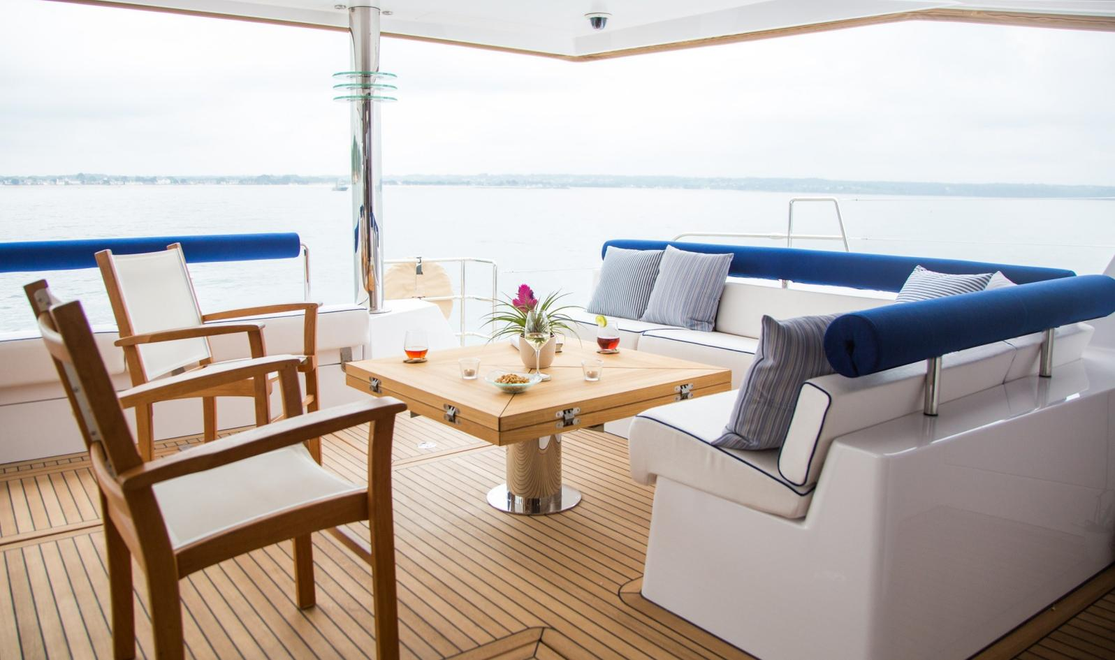
Again in order to keep the weight of the boat down, teak decking has been used only forward of the owners' cabin and in the aft cockpit.
